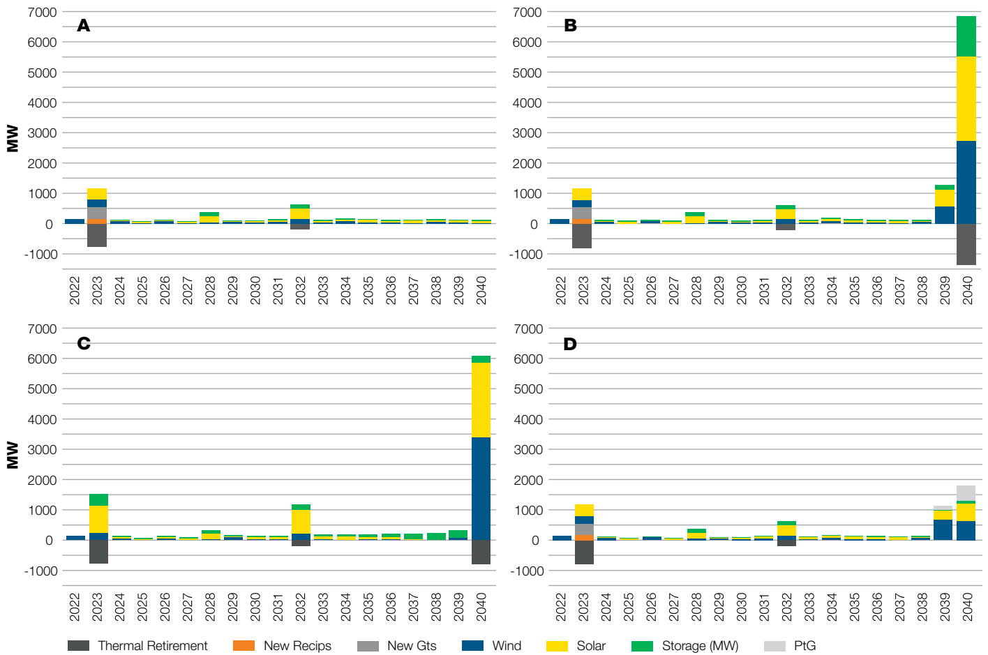
Figure 6.2-1. Annual capacity additions (and retirements) by Scenario. Cost-Optimal (A), 100% Carbon Free (B), 100% Carbon Free, no new thermal (C), 100% Carbon Neutral, with PtG (D)
